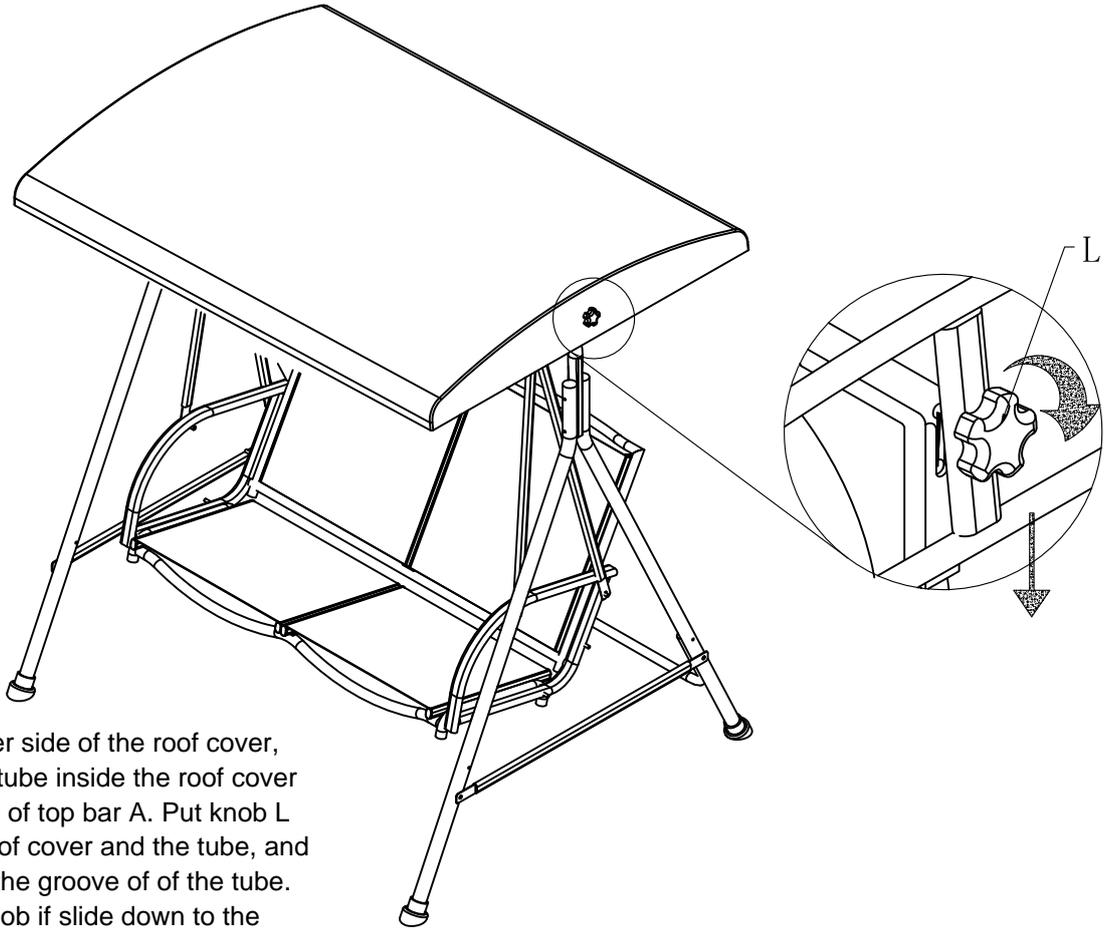
9. For the other side of the roof cover, pull down the tube inside the roof cover along the tube of top bar A. Put knob L through the roof cover and the tube, and slide down in the groove of the tube. Tighten the knob if slide down to the hole on the tube.
