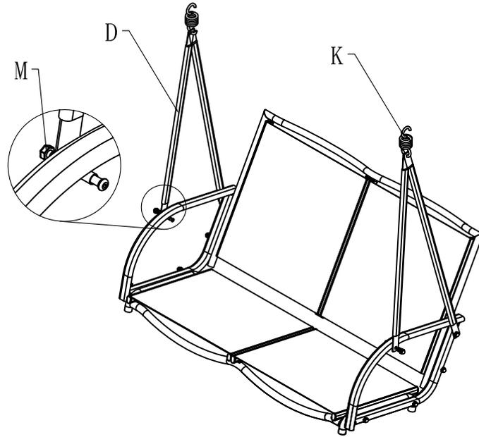
5. Assemble part D and part F with part M, and make the screws a little bit loose. Hang up part K.
