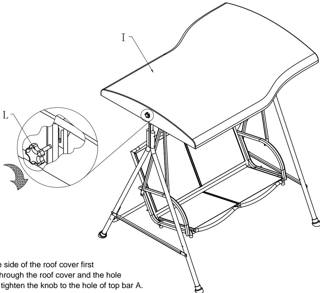
8. Install one side of the roof cover first
