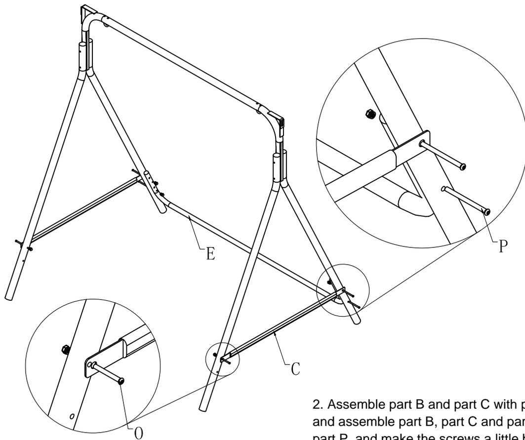
2. Assemble part B and part C with part O, and assemble part B, part C and part E with part P, and make the screws a little bit loose.
