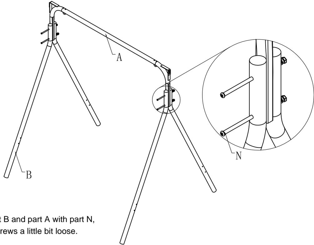
1. Assemble part B and part A with part N, and make the screws a little bit loose.
