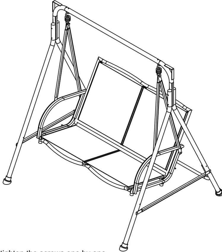
7. Swing the seat gently, tighten the screws one by one.
