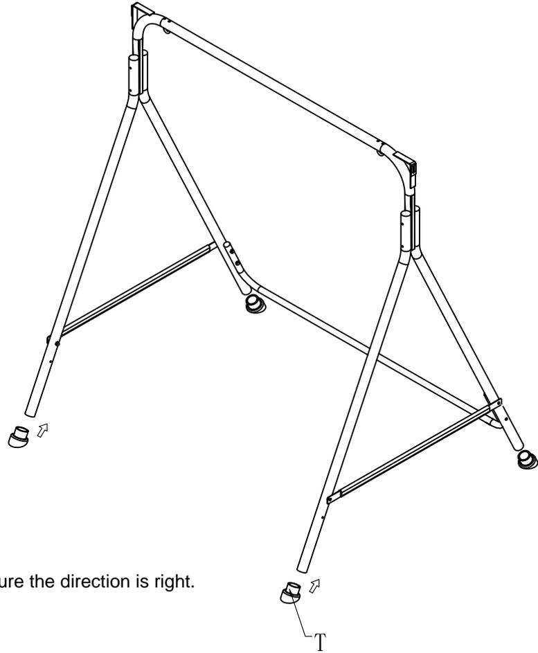
3. Assemble part T and make sure the direction is right.
